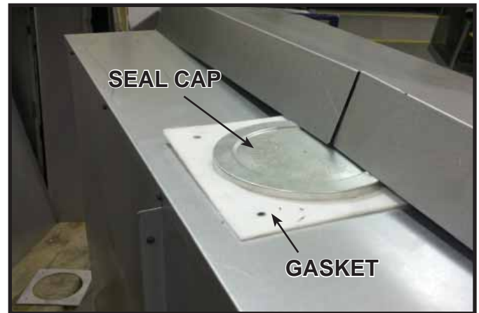
Figure 9.2 Seal Cap and Gasket Location
